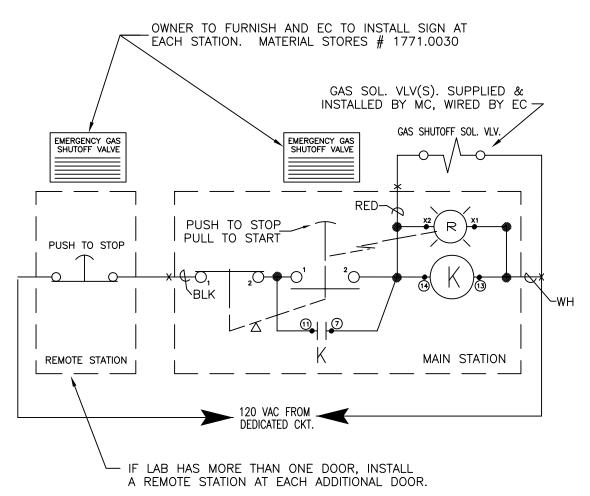
EC TO INSTALL BOXES, RACEWAY & WIRE. OWNER TO FURNISH PUSHBUTTONS ASSEMBLIES, FOR EC TO INSTALL & WIRE.
